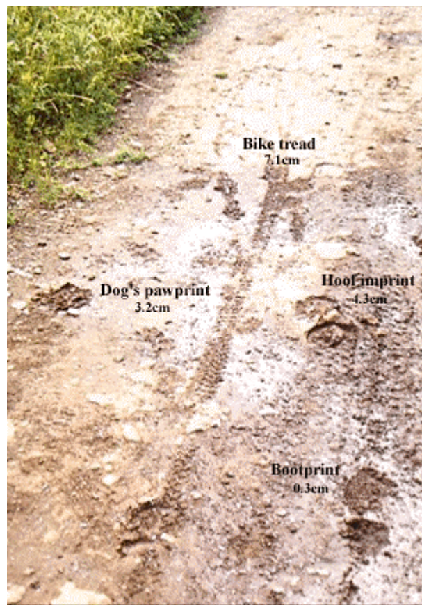
Fig 2.2 Depth measurements taken on Bulldog Motorway.
